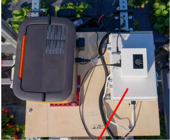
Edge computer, power supply and electronics box
