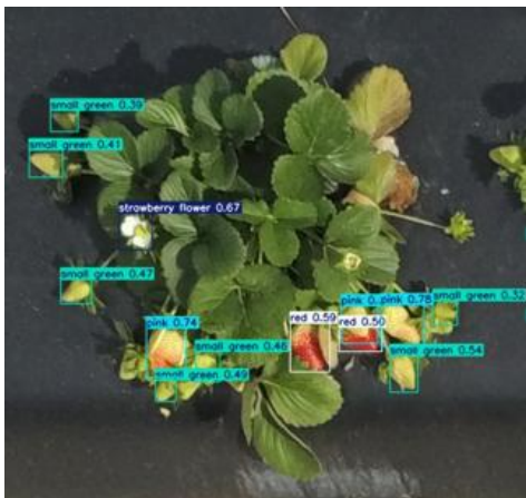
Figure 2. Example output from the YOLOv11 strawberry fruit and flower detection model using drone imagery. The system identifies strawberry flower (confidence 0.66–0.72), small green fruit (0.31–0.51), and pink fruit (0.76), illustrating accurate phenological detection under field conditions.
