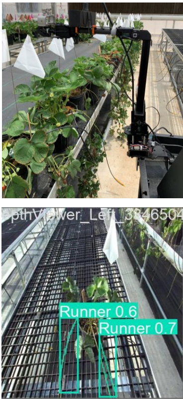
Figure 1. The setup of the AI-guided runner-cutting system in a controlled greenhouse environment. The upper image shows the robotic arm positioned beside strawberry rows, and the lower image displays the RGB camera's detection view with bounding boxes identifying runners and their confidence scores.
