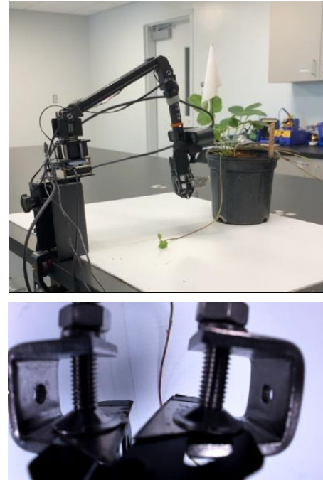
Figure 2. Laboratory demonstration of the robotic runner-cutting mechanism. The upper image shows the robotic arm aligning toward a detected runner on a potted strawberry plant, while the lower image presents a close-up of the dual-blade assembly during the cutting operation.
