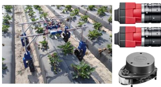
Figure 1. The ground vehicle with stereo vision cameras for capturing images of strawberry plants and LiDAR.
