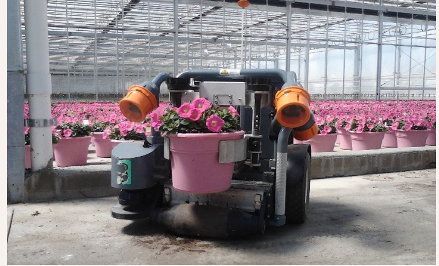
Harvest Automation's HV-100 ( https://www.public.harvestai.com/ ) for material handling for the Nursery and Greenhouse industry.
