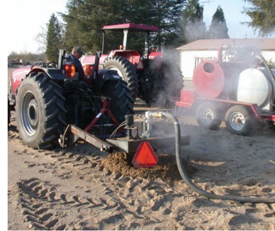
Soil steaming - tractor with a boiler that heats steam to more than 300 degrees F. Ten-inch spikes inject steam into the ground (Fennimore, UC)
