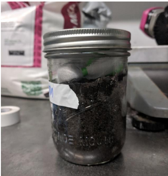
Figure 2. M. phaseolina inoculum placed on field soil inside mason jars and treated with different rates of 1,3-dichloropropene (Telone), chloropicrin (Pic) and their combination to simulate field applications.
