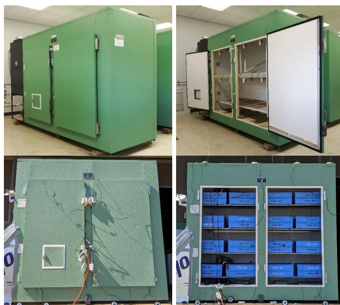
Figure 1. Plant sauna devices used for thermotherapy at the UF-GCREC (upper panels) and in nurseries in North Carolina and Canada (lower panels).
