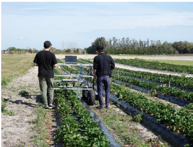
Figure 2. Programming navigation paths using the robot.
