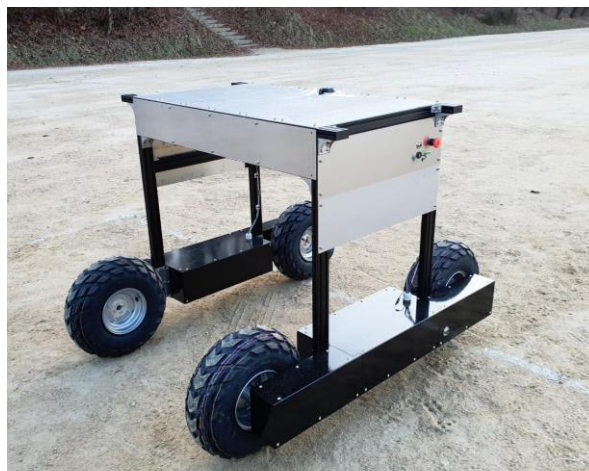
Figure 1. A four-wheel drive autonomous robot for this study donated by a company in Korea.
