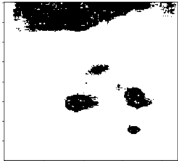
Figure 5. Thermal to binary image conversion. Black spots are water droplets.
