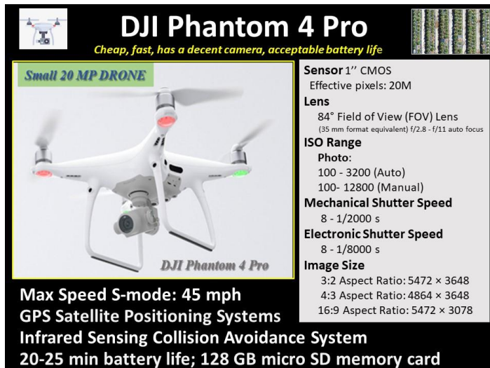
Figure 2. A DJI Phantom 4 Professional Series drone.
