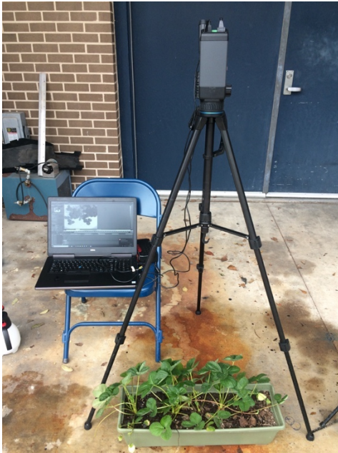
Figure 2. Thermal camera setup for lab experiments.
