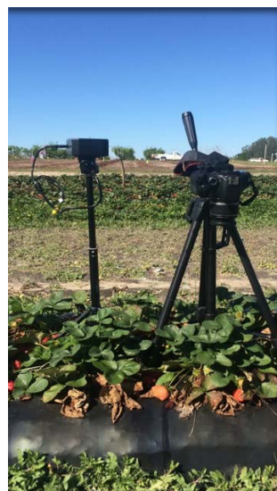
Figure 1. Thermal (left) & color (right) camera setup for field imaging.
