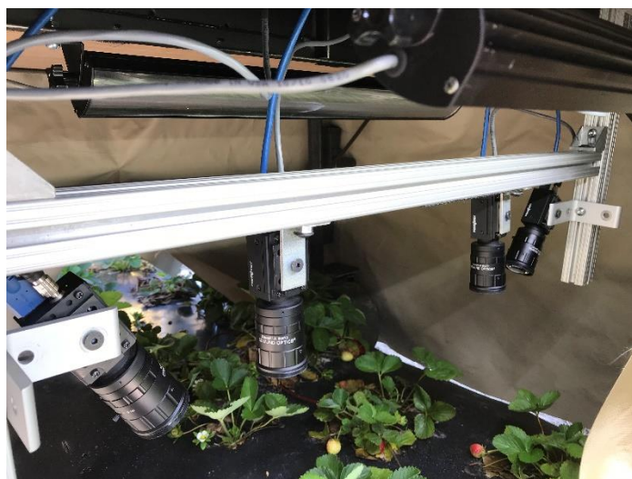
Figure 1. Camera and light arrangement for imaging.
