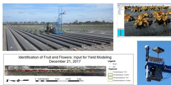
Clockwise from top left: imaging platform collecting data in the field, 3d point cloud model of strawberry canopy viewed in Agisoft Photoscan, imaging platform showing GPS and camera suite, intermediate step in modeling process showing input of fruit and flowers for specific dates and treatments on a specific date as input for yield model.
